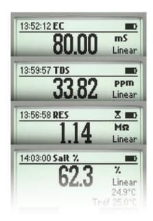
• EC, TDS, resistivity and salinity measurements in one meter
